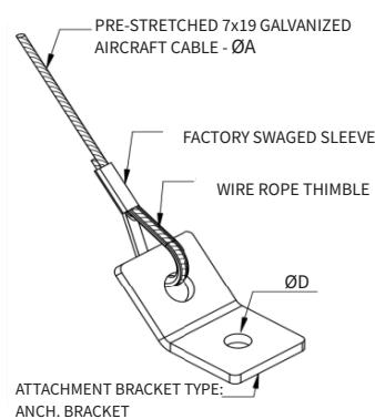
OPTION: 1 CABLE ASSEMBLY WITH ANCH. BRACKET
