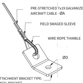
OPTION: 2 CABLE ASSEMBLY WITH RETROFIT BRACKET
