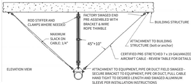
**CABLE RESTRAINT INSTALLATION WITH VIBRATION ISOLATOR**
