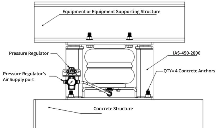
9. Loosen the two **Lock Nuts** located inside each stanchion as shown in the picture and move it down to have 1/4" to 3/8" gap between washer and bottom of **Isolator Reinforced Neoprene Snubber** on both sides
