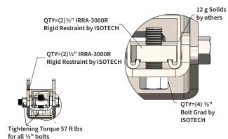
NutTeeth grip channel's inturned edges, tying the channel sides together in a "box" configuration for added strength
