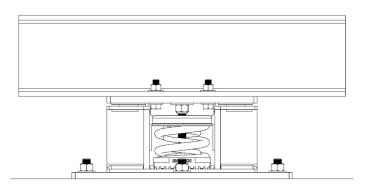
7. Ensure isolator top plate is fully covered by equipment and/or equipment supporting structure as shown in pictures below. For installations where less than 80% of isolator top plate is covered, refer to Step 11 shown on the third page:
