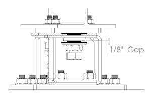
8. Loosen the two Lock Nuts located inside each stanchion as shown in the picture and move it down to have 1/8" gap between washer and bottom of Reinforced Rubber Washer
