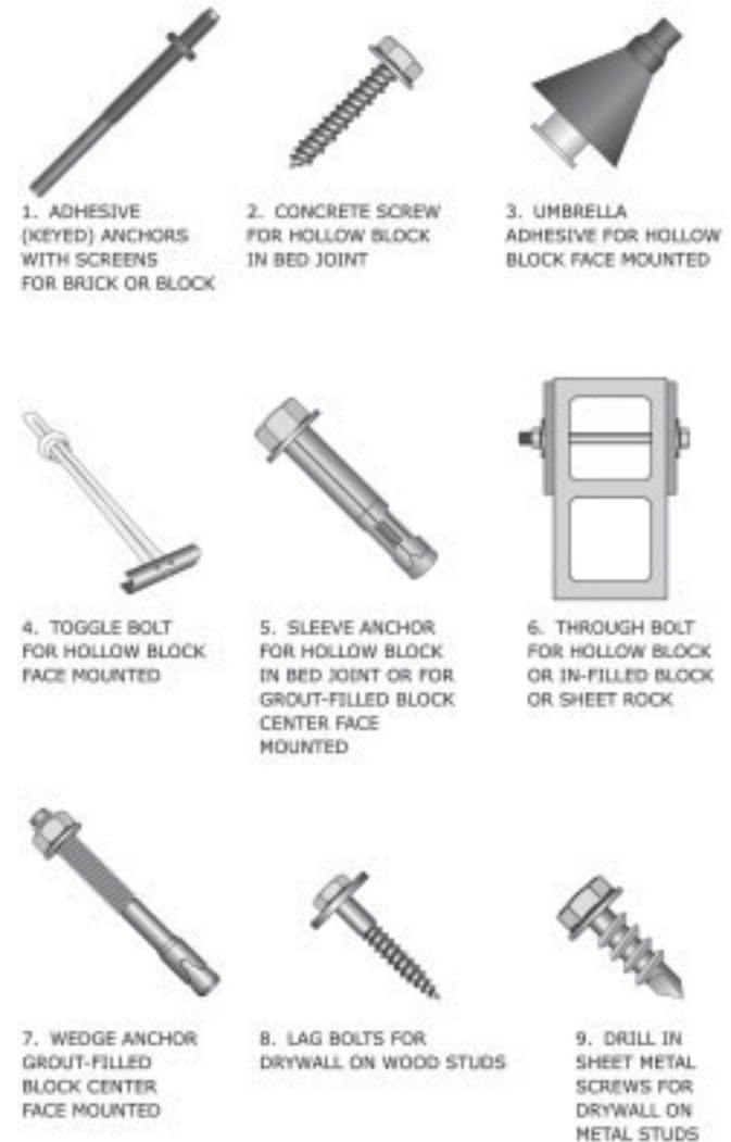
Figure 117: Types of masonry and drywall anchors.
