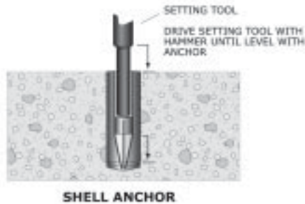
Figure 111: Set shell anchors.
