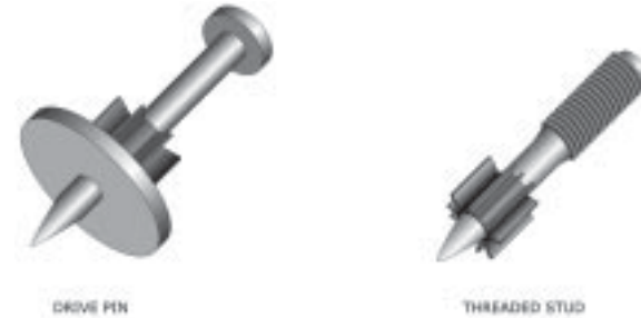
Figure 123: Two types of power-actuated anchors.
