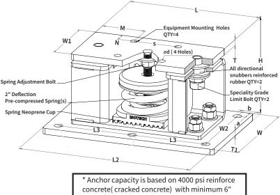
Anchor capacity is based on 4000 psi reinforce concrete( cracked concrete) with minimum 6" edge distance. Hilti anchors- Type KBTZ - were considered for all calculations. Detailed calculations must be performed if different anchors are used.
