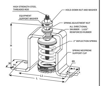
\* Anchor capacity is based on 4000 psi reinforce concrete( cracked concrete) with minimum 6" edge distance. Hilti anchors- Type KBTZ - were considered for all calculations. Detailed calculations must be performed if different anchors are used.
