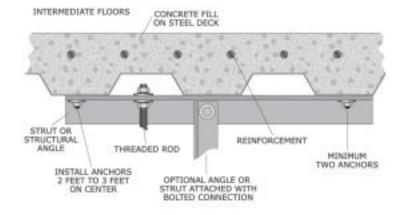
Figure 93: Cast-in-place anchor; concrete fill on steel deck.
