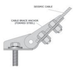
Figure 150: Cable attached with bolts to a bracket.
