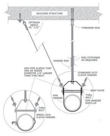
Figure 64: Single clevis hanger support with cable lateral supports at the restraining bolt.
