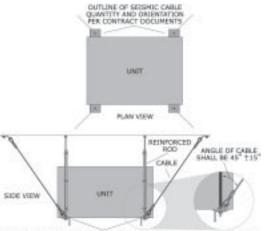
PREINSTALLED BRACKETS OR EQUIPMENT SUPPORT FRAMING ANGLED VIEW
