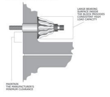
Figure 142: Umbrella anchor in a hollow block wall.
