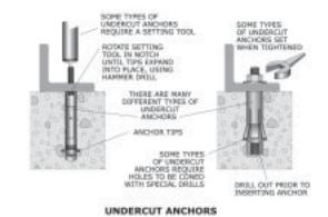
Figure 133: Set undercut anchors.
