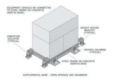
Figure 120: Typical installation of open isolators and snubbers.
