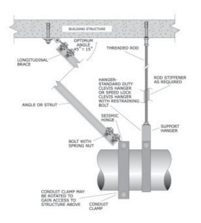
Figure 68: Conduit clamp supports with longitudinal strut or angle lateral support and hanger rod.
