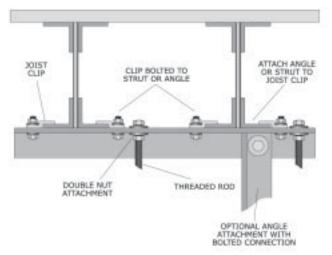
Figure 97: Bar joist construction.
