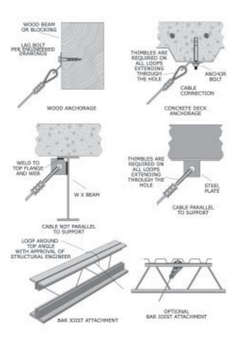
Figure 100: Attachments to the building structure.
