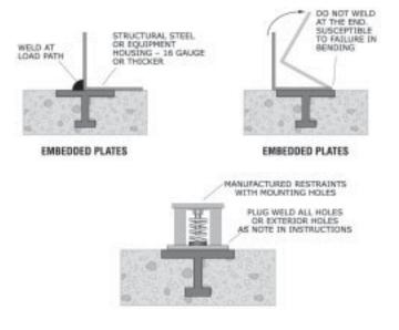
Figure 148: Welding to embedded plates.
