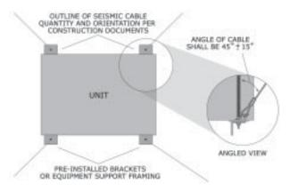
Figure 105: Plan view of vibration isolation suspended attachment to the building structure.
