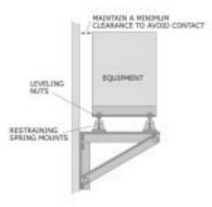
Figure 126: Wall-mounted, vibration-isolated equipment.
