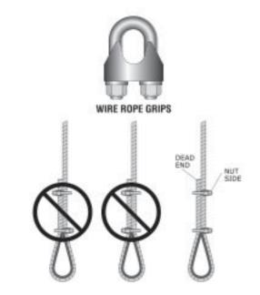
Figure 153: Wire rope grip assemblies.
