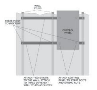
Figure 157: Direct attachment of a strut assembly support to wall.
