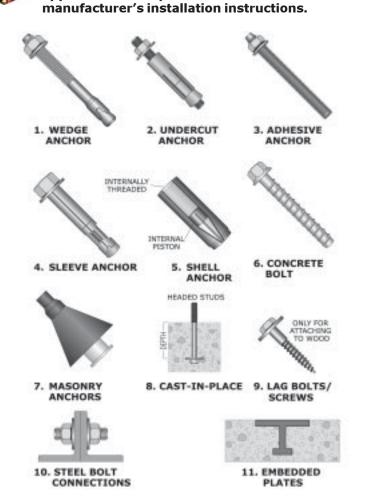
Figure 127: Types of anchors.
