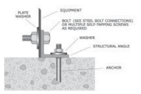
Figure 135: Installing a reinforcing angle bracket to equipment.
