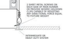
Figure 162: Typical ways to attach light fixtures in suspended T-bar ceiling.
