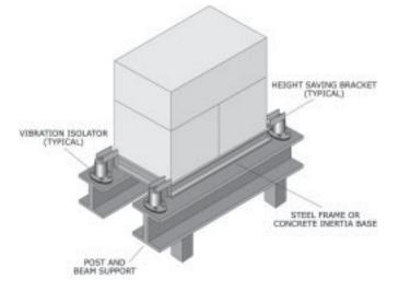
Figure 91: Equipment attached using restrained vibration islators on a post and beam support.
