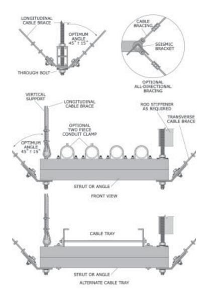
Figure 71: Trapeze support with cable lateral supports.
