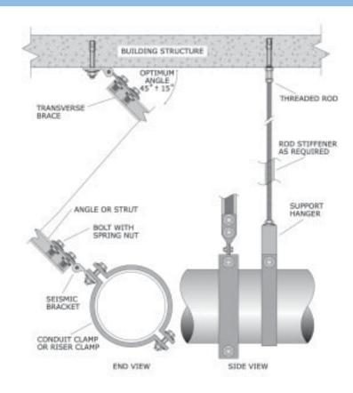
Figure 67: Conduit clamp supports with transverse strut or angle lateral support and hanger rod.
