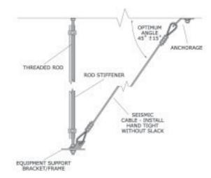
Figure 101: Attachment of cable to the equipment.
