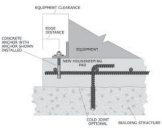
Figure 159: Housekeeping pad in section view.
