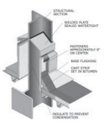
Figure 88: Flashing around a stanchion.
