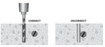
Figure 130: Drilling into concrete with rebar.
