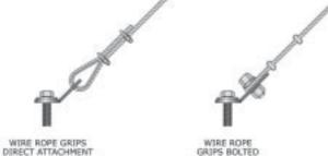
Figure 149: Cable attachments.
