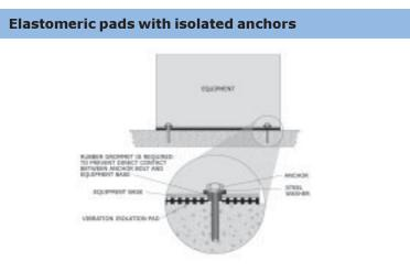
Figure 122: Elastomeric pads with isolated anchors.
