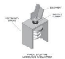
Figure 119: Attachment of equipment to restrained vibration isolators.
