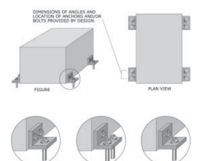
ONE ANCHOR AND TWO BOLTS TO EQUIPMENT IS OK
