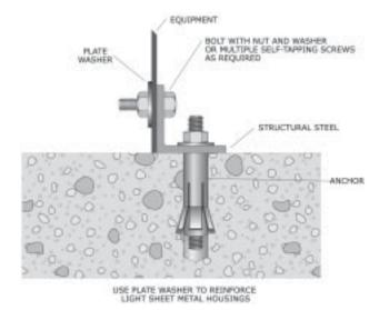
Figure 145: Bolting equipment to an angle.
