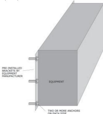
Figure 123: Direct attachment to a wall.
