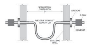
Figure 72: Seismic joint.
