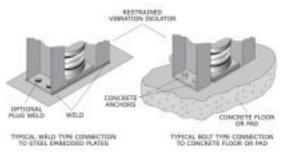
Figure 118: Attachment of restrained vibration isolators to the building structure.
