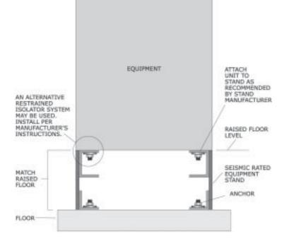
Figure 84: Electrical equipment installed on a raised floor.
