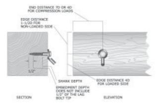
Figure 137: Spacing requirements for wood lag bolts.
