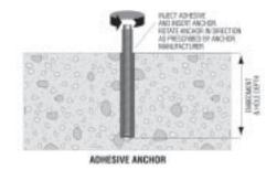
Figure 131: Adhesive anchor installation.
