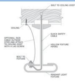
Figure 163: Pendant light fixture attachment
