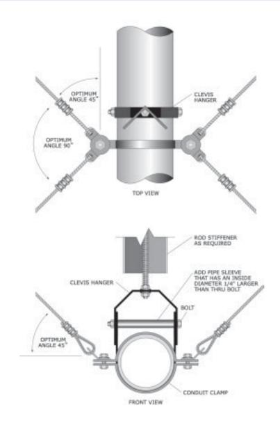
Figure 66: Single clevis hanger with four-way cable brace.
