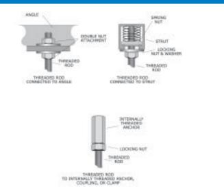
Figure 147: Attaching the top connection of the treaded rod.
