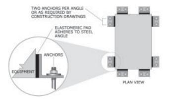
Figure 82: Equipment installed with bumpers.
