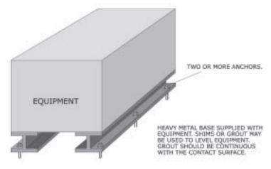
Figure 75: Direct attachment of equipment with structural steel frame or base to a building.
