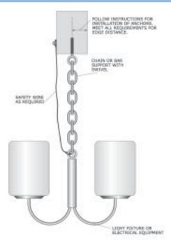
Figure 110: Chain mounted or bar support with swivel.
