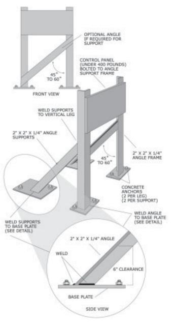
Figure 156: Angle assembly support from floor.
