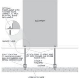
Figure 86: Equipment bolted beneath a raised floor.
