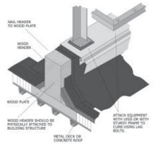
Figure 90: Attachment of equipment to a wood frame.
