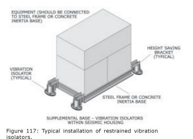
More than four restrained vibration isolators
