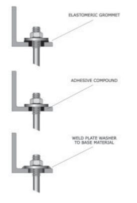
Figure 76: Three options to repair oversized holes.
